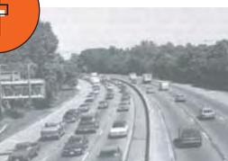
**LOS F** – Represents the worst conditions with heavily congested flow and traffic demand exceeding capacity, characterized by stop-and-go waves, poor travel time, low comfort and convenience, and increased accident exposure.
