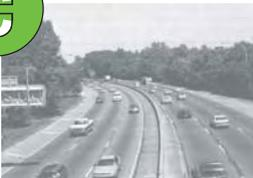
**LOS C** – Represents a constrained constant flow below speed limits, with additional attention required by drivers to maintain safe operations. Comfort and convenience levels of the driver decline noticeably.
